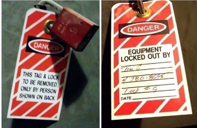
Figure 4.10 – Typical lock and tag-out system.
